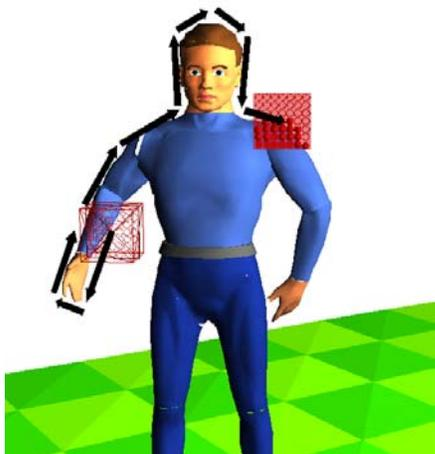
Figure 3: Tracing objects to estimate shape and size using the proximity-space method.
