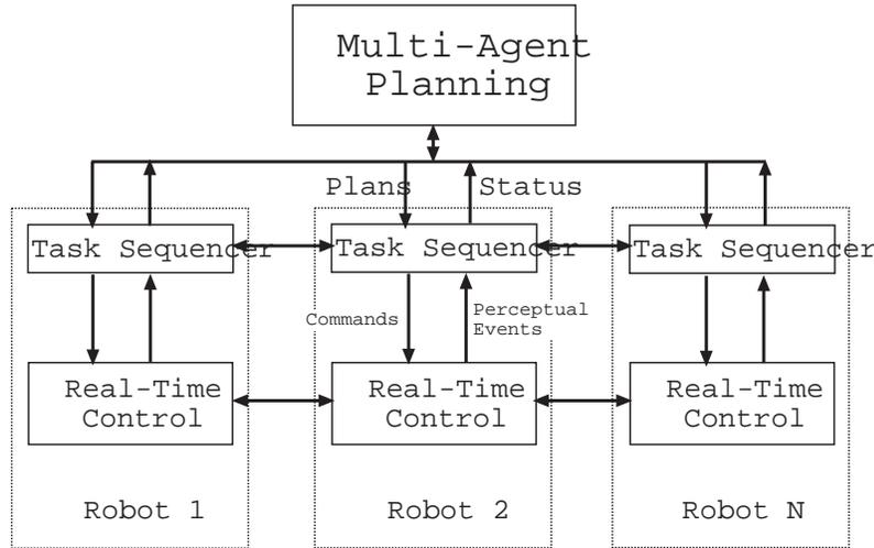
**Fig. 1.** A distributed, multi-layered robot architecture.
