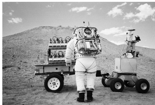
Figure 2: The suited test subject retrieves a geophone from the trailer, pulled by ERA.
