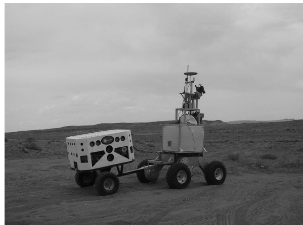
Figure 3: ERA pulls IHOPP, which provides all power to the robot.
