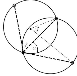
Figure 5: CARMEL's three object triangulation using the circles method.
