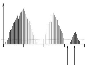
Figure 2: The Polar Histogram has “mountains” in the direction of obstacles. VFH steers the robot toward a “valley” in the direction of the target.
