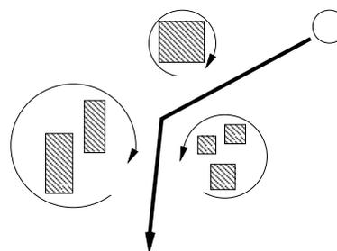
Figure 3: In NaTs each obstacle or group of obstacles is spun. The spin tells the robot to which side of the obstacle it should pass.
