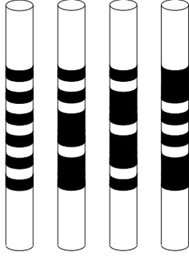
Figure 4: Example object tags showing the basic pattern and objects with bit pattern of 0, 5, 10 and 17.
