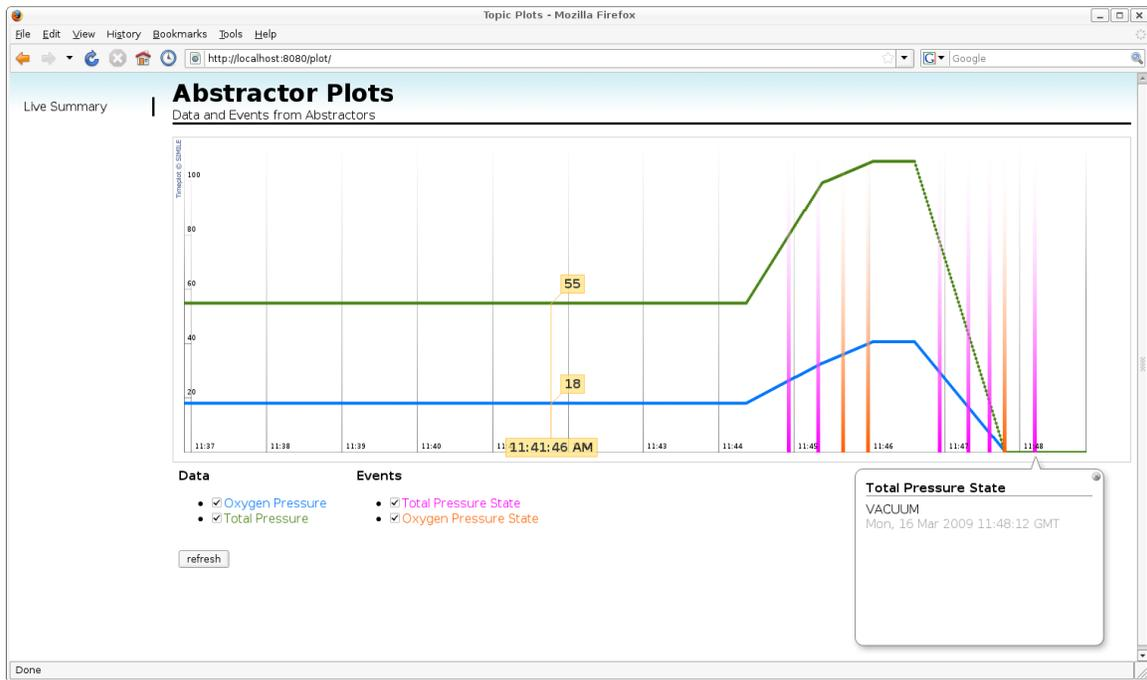
Figure 7. Graph of events and data during the airlock’s readying for EVA
