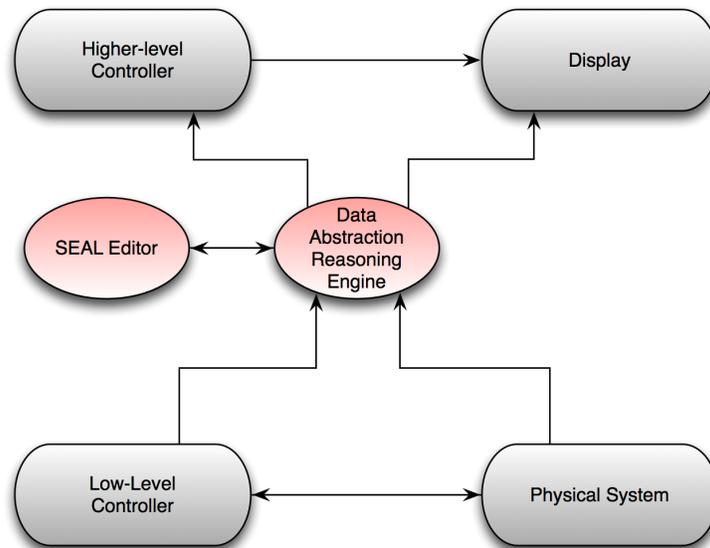
Figure 1. General overview of the Data Abstraction Architecture for Spacecraft Autonomy
