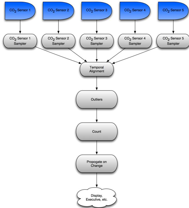
Figure 4. A data abstraction network for detecting a carbon dioxide sensor failure.
