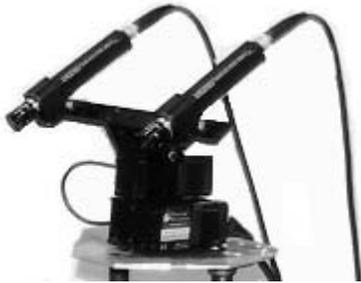
Figure 3: The vision system cameras and head.
